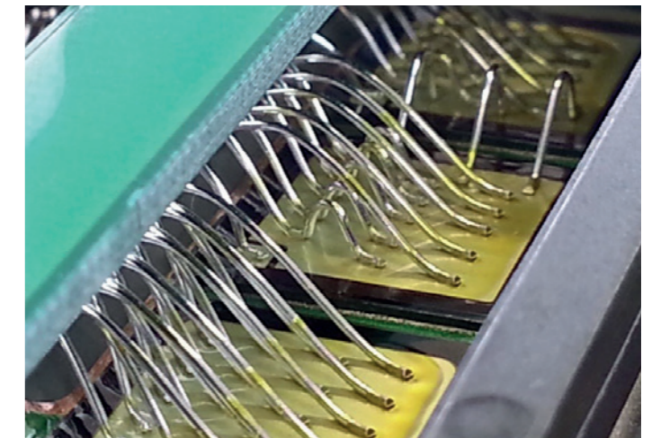
Fig. 5 Stich-bond layout and improved bonding parameters boost the power cycling capability
