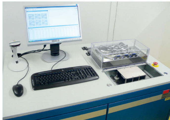
Baseplate flatness tester. Mechanical measurement under pressure (resolution up to 0.1 micrometer)
